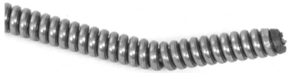
Figure 15 – Bend At Cable End
