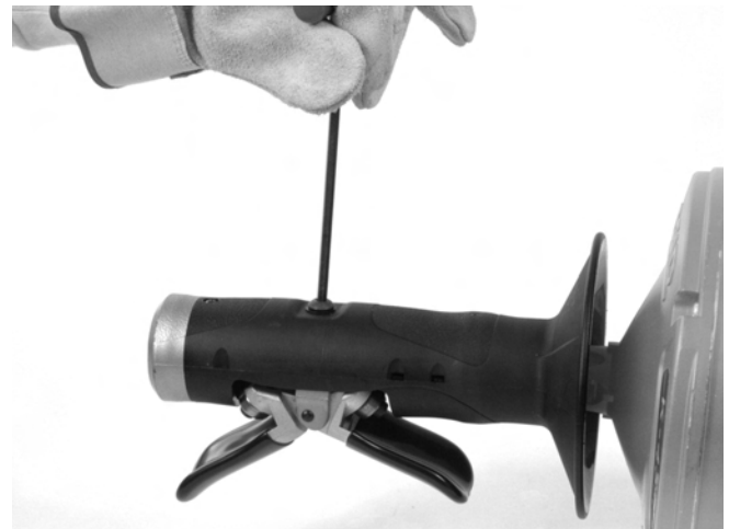
Figure 12A – Removing AUTOFEED Screw
