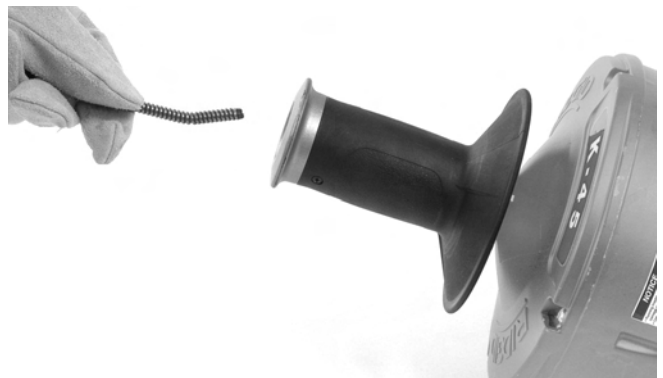
Figure 17 – Loading Cable Without Changing Inner Drum
