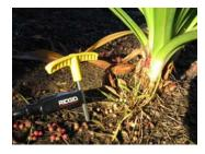
Dry sandy soil provides more of a challenge. In dry, sandy soil the resistance to current flow causes a lower locatable signal. Water can be added to very dry soil to improve the grounding and lower resistance. Keep a mixture of Gatorade and Water in your vehicle for this purpose.
