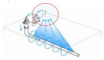
From the transmitter, down the line, back through the dirt it then needs to complete the circuit to the transmitter.
